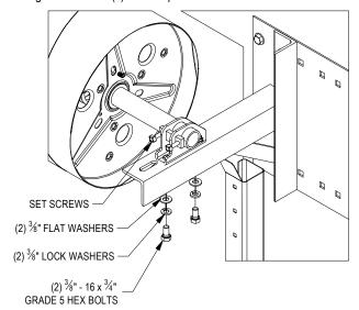
FIGURE 14: SECURING SADDLE
