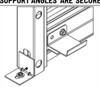
STEP 1: Install the Mini Handle to the bottom bar on latch side of door using (2) 1/4" - 20 x 3/4" Carriage bolts and (2) 1/4" - 20 Wiznuts.
