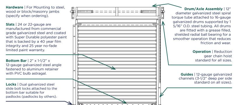
The **Model 300 Rolling Steel Slat Door** with nylon end locks and 12-gauge roll formed guides is an economical alternative slat door that is easy to maintain and service. The curtain is pre-assembled on the drum at the factory making the installation easier and faster.
